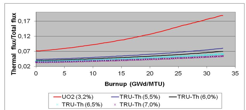
**Figure 3 - The hardening spectrum during the burnup**
